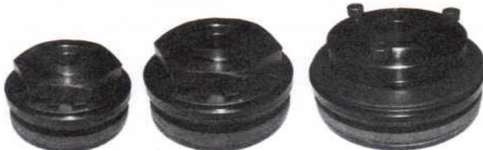
Benwan torque limiter is a protective device which limits the torque transmitted in a drive system by slipping when the demanded torque exceeds a preset value as a result of shock loads, overloads or machine jams. It will automatically reengage when the overload is removed. No resetting is required.
